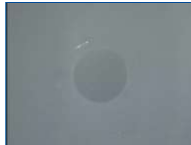
Improperly Keyed APC Connector
